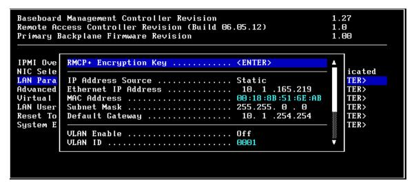
Once the 'IPMI over LAN' and 'LAN Parameters' options have been configured, hit <ESC> to exit the configuration window; the system could ask if you wish to save the changes. If so, select Yes to continue the boot up process.
